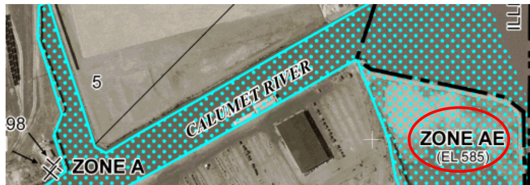
➔ Limits of coastal flood effects from Lake Michigan are shown on the FIRM (white line)
